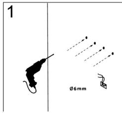
For drywall installation, mark the hole locations and drill  $\Phi$  6mm holes for the drywall anchors. Install a junction box behind the mirror for power connections.
